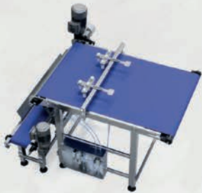
Damaged Dough selector
